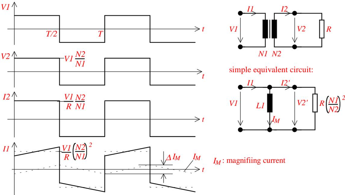
Figure 5.2.1: Voltages and currents at a transformer
