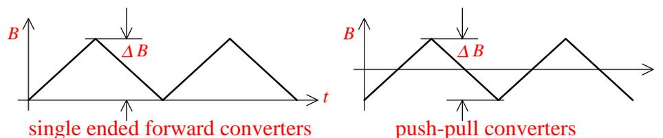
The calculation of the minimum number of turns  $N_{1\min}$  is equal for these different types of switch mode power supplies.
