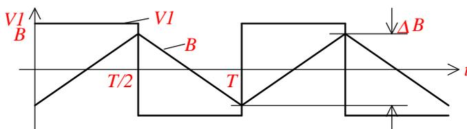
Figure 5.2.2: input voltage and magnetic flux density at the transformer
